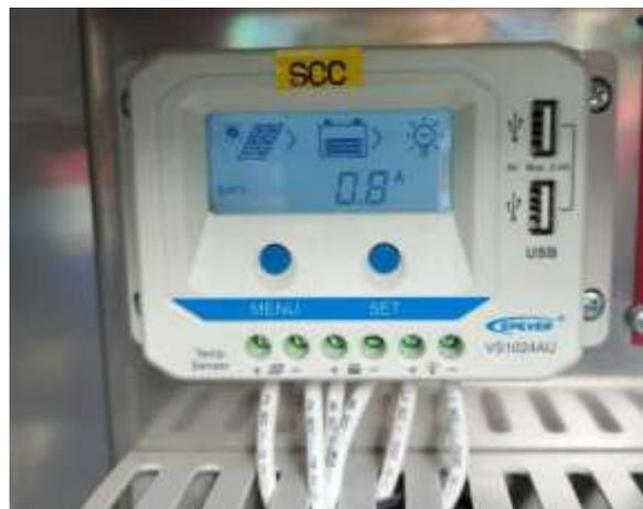
Gambar 5. Perangkat SCC (Solar Charge Controller)
