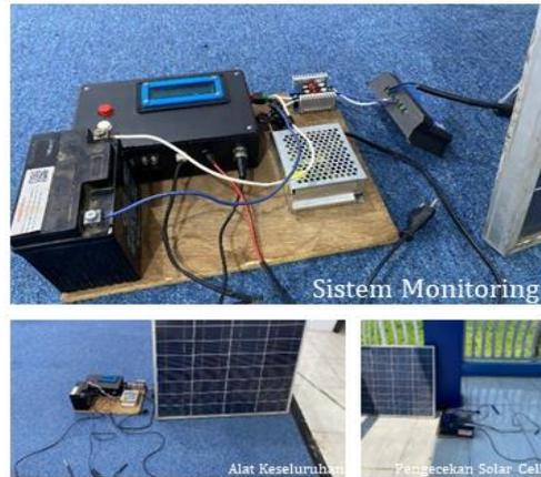
Gambar 5. Alat Sistem Monitoring Kualitas Air Kolam Ikan Lele Berbasis IOT
