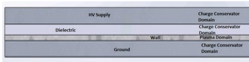
Fig. 4. Simulation boundary conditions for ozone plasma generation.
